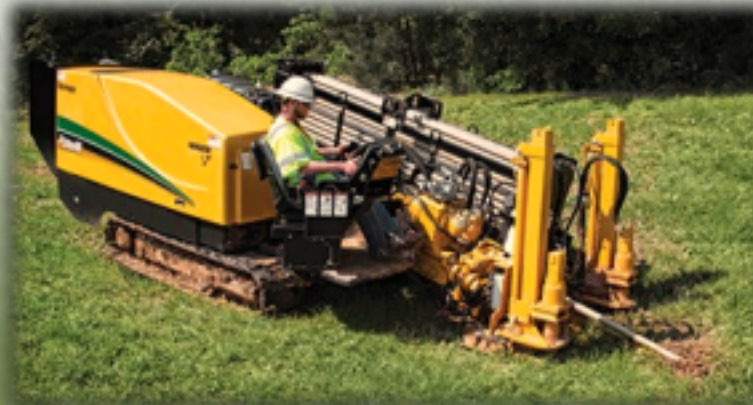
Buried Cable Placement (Directional Bore)
