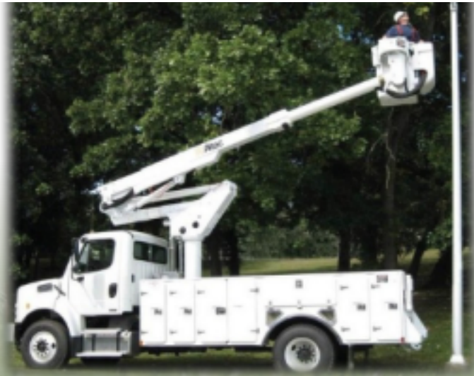
Aerial Cable Placement (Bucket Truck)
